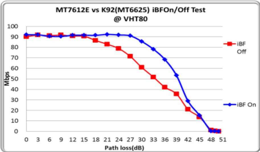
Below is an illustration of the performance in an office setting. The blue indicates the improvement provided by MediaTek's solution.
