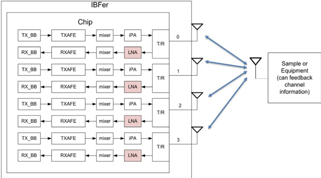
If the iBF Calibration is perfect, the TX and RX paths are reciprocal, and iBF can achieve similar performance as with EBF. Here, we use a VHT80 throughput as an example. However, the perfect iBF calibration needs more factory calibration time. MediaTek can provide the trade-off solution between iBF calibration time and the acceptable iBF gain.
