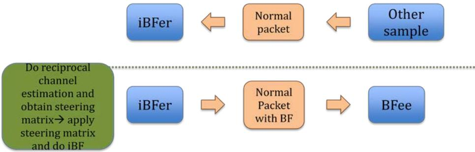
Each device needs to perform iBF Calibration only once in the factory, thereby enabling the BF gain even for the 11a (Legacy) device.
